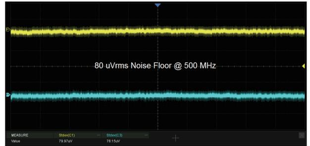
Low noise floor: Only 80  $\mu$ V rms at 500 MHz bandwidth.
