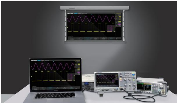
With 100 Mbps LAN, the internal web page can update at a rate of up to 10 times/s, providing a nearly-real time update of waveform data and measurements. When viewed on a PC, the screen can be displayed in full screen mode. With this feature and a PC VGA interface, you can easily use a projector or other video display device to deliver the screen information to a larger audience.
