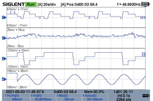
The measurement Logger is the mode of logging the measurement value for a long time. For the amount of measurement data is relatively small, to process quickly, the data is logged in memory. After stopping logging, the data can be saved into the internal flash or external U disk.
