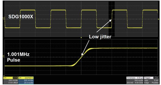
When a Pulse waveform is generated by a common DDS generator, there will be a one-clock-jitter if the sampling rate is not an integer-related multiple of the output frequency. SDG1000X EasyPulse technology successfully overcomes this weakness in DDS designs and helps to produce low jitter Pulse waveforms.
