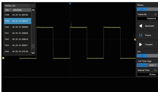
History function can record up to 80,000 frames of waveforms. The recording is executed automatically so that the customer can playback the history waveforms at any time to observe unusual events and quickly locate the area of interest using the cursors or measurements. The failed frames of the Mask Test can be stored as history
