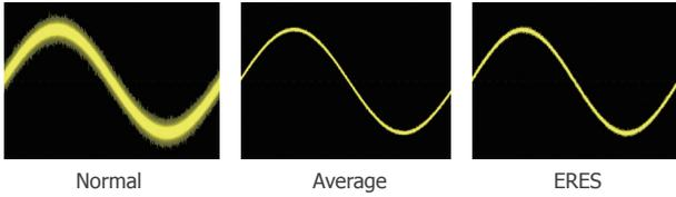
Average and ERES (Enhanced Resolution) acquisition modes are hardware-based, allowing the waveforms to be captured at a faster rate
