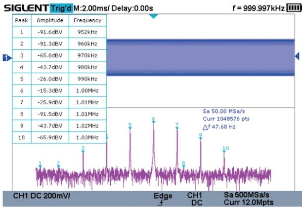
The new math co-processor enables FFT analysis of incoming signals using up to 1 M samples per waveform. This provides high-frequency resolution with a fast refresh rate. The FFT function also supports a variety of window functions so that it can adapt to different spectrum measurement needs. Support Peaks, Markers, a variety of numbers.
