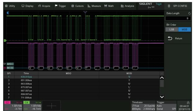
In addition to the decoder lanes correlated to the waveform, bus protocol information can be displayed in tabular form. I2C, SPI, UART, CAN, LIN, CAN FD, FlexRay, I2S and MIL-STD-1553B are supported.
