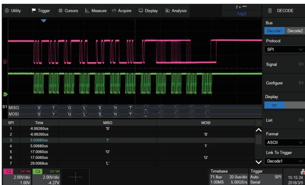
Display the decoded characters through the events list. Bus protocol information can be quickly and intuitively displayed in tabular form. I2C, SPI, UART, CAN, LIN, CAN FD, FlexRay and I2S and MIL-STD-1553B are supported
