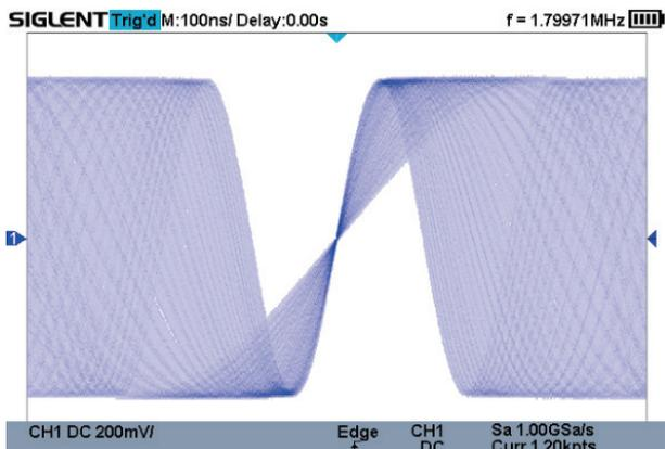
SPO display technology provides fast refresh rates. The resulting intensity-graded trace is brighter for events that occur with more frequency and dims when the events occur with less frequency.
