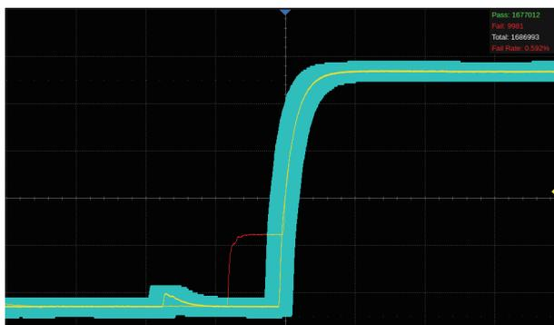
The oscilloscope utilizes a hardware-based Mask Test function, performing up to 14,000 Pass / Fail decisions each second. It is easy to generate user-defined test templates to provide trace mask comparisons, making it suitable for long-term signal monitoring or automated production line testing
