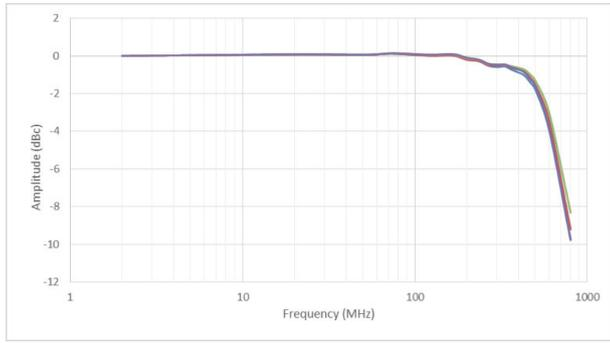
500 MHz bandwidth (at 2 GSa/s sample rate with 500 MHz bandwidth option).
