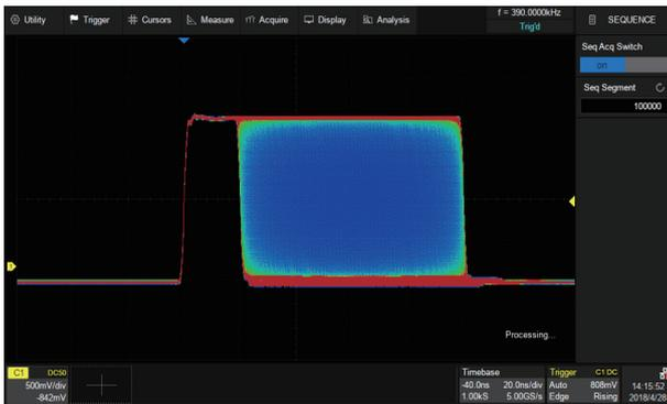
Segmented memory collection will store the waveform into multiple memory segments (up to 100,000) and each segment will store a triggered waveform as well the dead time information. The dead time between segments can be as small as 2 μs. All of the segments can be played back using the History function
