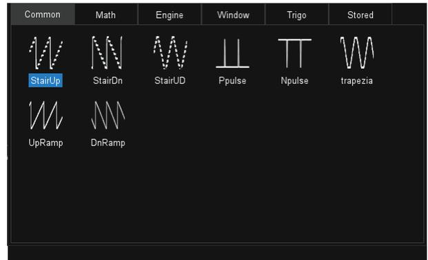
The built-in waveform generator can output waveforms with up to 25 MHz frequency and  $\pm 3$  V amplitude. Six basic waveforms together with multiple types of predefined waveforms and as user-defined arbitrary waveforms are supported
