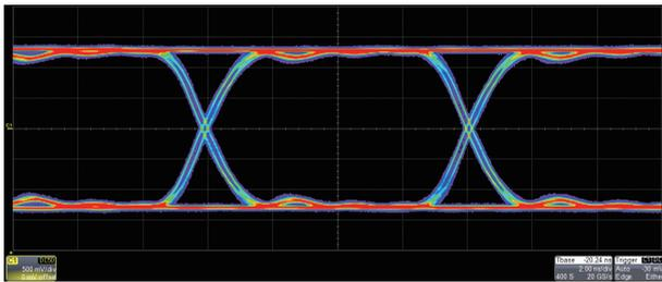
PRBS3 ~ PRBS32 with finely adjustable  $10^6$  bps ~ 300 Mbps bit rate and 1 ns ~ 1us edge.
