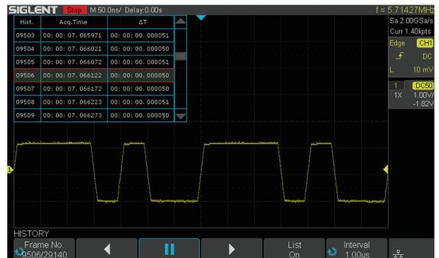
Playback the latest triggered events using the history function. Segmented memory collection will store trigger events into multiple (Up to 80,000) memory segments, each segment will store triggered waveforms and timestamp of each frame.
