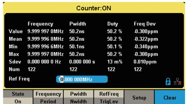
8-digit hardware frequency counter with statistics function and input range of 0.1 Hz ~ 400 MHz.
