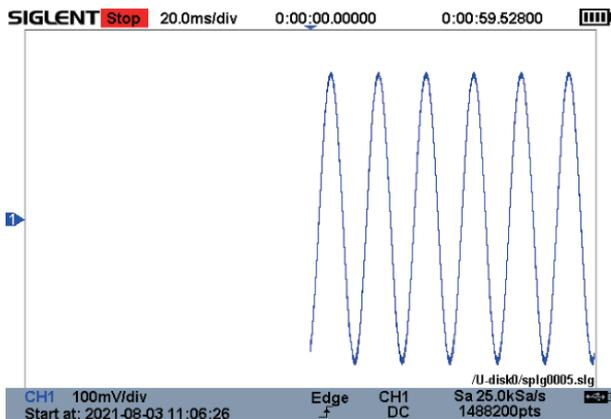
The Sample Logger is the mode of logging the sampling points for a long time. For there are many sampling points to log, they are logged into the internal flash or external U disk in real-time. After stopping logging, the user can recall the sampling points on the oscilloscope, or analyze the saved data on the computer.
