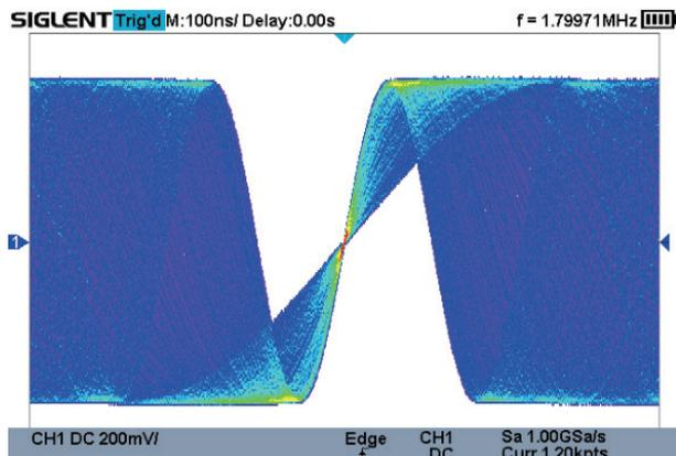
The color temperature display is similar to the intensity-graded trace function, but the trace occurrence is represented by different colors (color "temperature") as opposed to changes in the intensity of one color. Red colors represent events that occur more frequently, while blue is used to mark points that occur less frequently.
