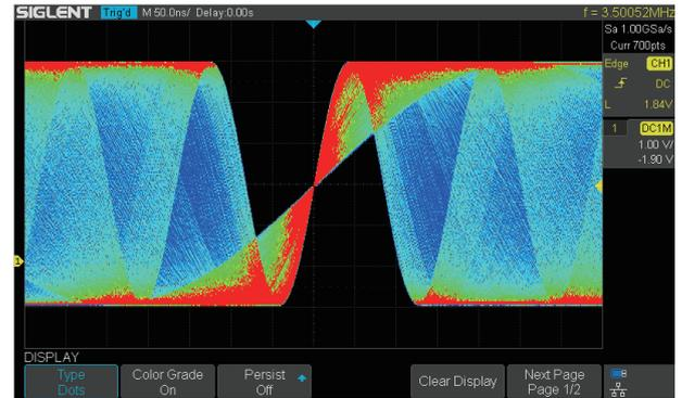
The color temperature display is similar to the intensity-graded trace function, but the trace occurrence is represented by different colors (color "temperature") as opposed to changes in the intensity of one color. Red colors represents the more frequent events, while blue is used to mark points that occur less frequently.
