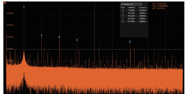
Hardware-accelerated FFT supports up to 8 Mpts operation. This provides high-frequency resolution with a fast refresh rate. The FFT function also supports a variety of window functions so that it can adapt to different spectrum measurement needs. Three modes (Normal, Average, and Max hold) can satisfy different requirements for observing the power spectrum. Auto peak detection and markers are supported.
