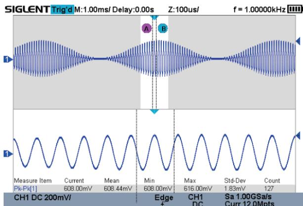
Through Gate and Zoom measurement, the user can specify an arbitrary interval of waveform data analysis and statistics. This helps avoid measurement errors that can be caused by invalid or extraneous data, greatly enhancing the measurements' validity and flexibility.
