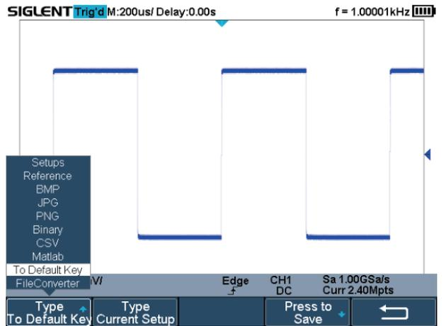
The current parameters of the oscilloscope can be preset to Default Key through the Save menu.
