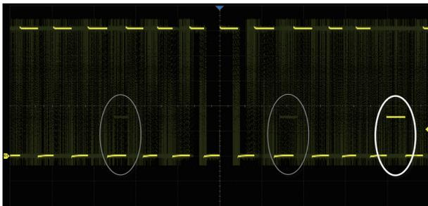
With a waveform update rate of up to 100,000 wfms/s, the oscilloscope can easily capture unusual or low-probability events. In Sequence mode, the waveform capture rate can reach 500,000 wfms/s
