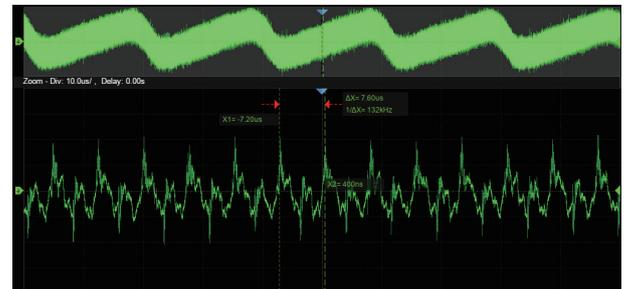
Using hardware-based Zoom technique and record length of up to 200 Mpts, users can select a slower timebase without compromising the sample rate, and then quickly zoom in to focus on the area of interest
