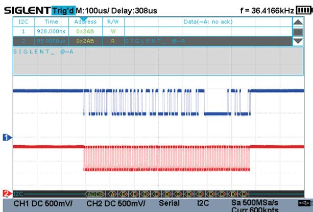
SHS800X/SHS1000X displays the decoding through the events list. Bus protocol information can be quickly and intuitively displayed in a tabular format.
