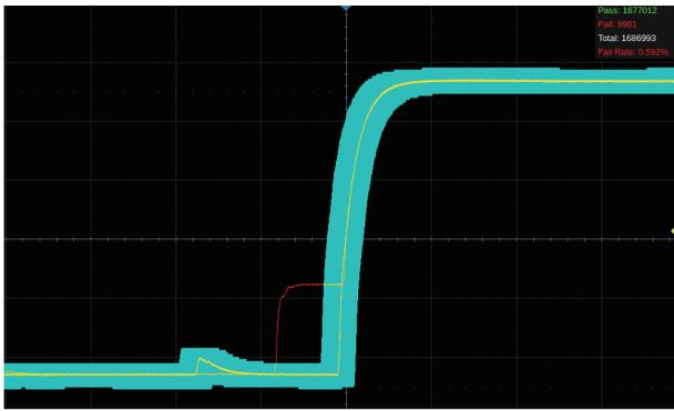
The oscilloscope utilizes a hardware-based Mask Test function, performing up to 18,000 Pass / Fail decisions each second. It is easy to generate user-defined test templates to provide trace mask comparisons, making it suitable for long-term signal monitoring or automated production line testing
