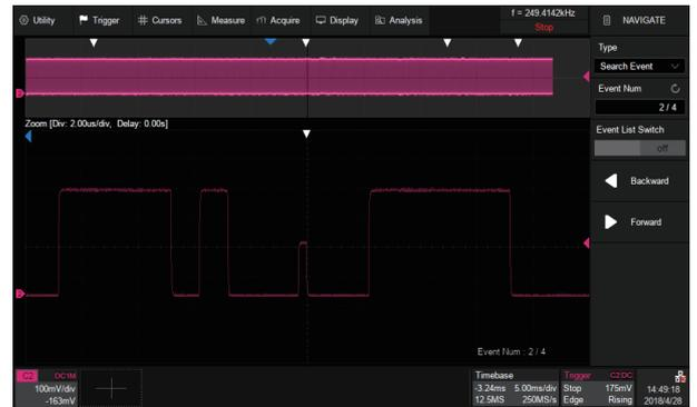
The SDS5000X can search events specified by the user in a frame. Events flagged by the Search can be recalled automatically using Navigate. It can also navigate by time (delay position) and history frames
