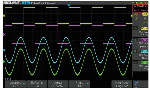
The four channel series has two 1 GSa/s ADC chips (channel 1 and 2 share one, channel 3 and 4 share another), so that each channel can achieve sample rates up to 500 MSa/s and work on bandwidths of 200 MHz when all channels are enabled.
