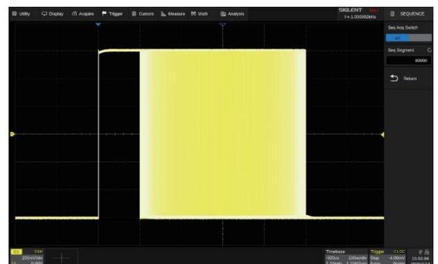
Segmented memory collection will store the waveform into multiple memory segments (up to 80,000) and each segment will store a triggered waveform as well as the dead time information. The interval between segments can be as small as 1.3µs. All of the segments can be played back using the History function
