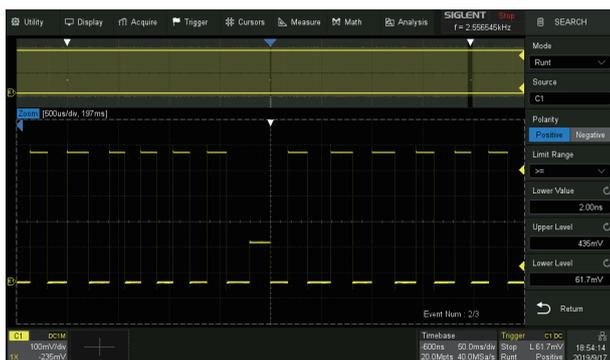
The oscilloscope can search events specified by the user in a frame. Events flagged by the Search can be recalled automatically using Navigate. It can also navigate by time (delay position) and history frames
