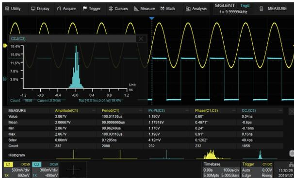
Statistics shows the current value, maximum value, minimum value, standard deviation and mean value of up to 5 parameters. Histogram is available to show the probability distribution of a parameter
