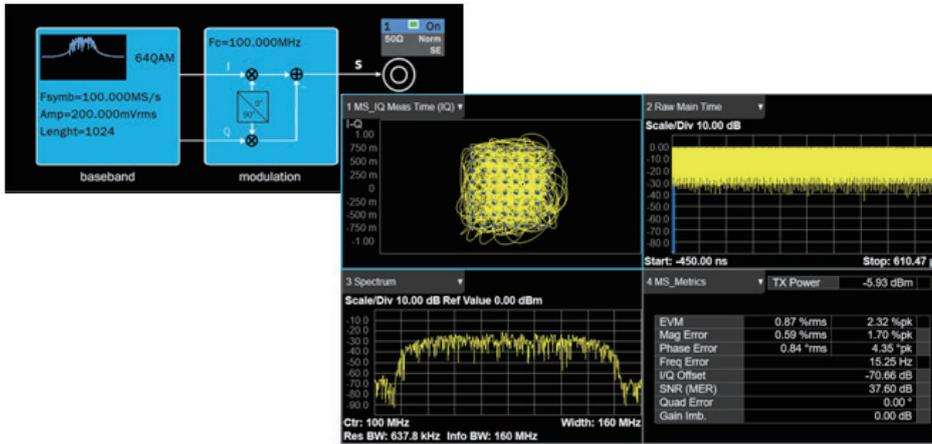
The SDG7000A can generate common modulation types of IQ signals, such as ASK, FSK, PSK, QAM. With the innovative resampling technology, excellent EVM performance can be obtained at any symbol rate between 250 S/s ~ 500 MS/s. The built-in digital quadrature modulator can modulate the carrier of the IQ signal to any frequency between 0 Hz~1 GHz. The EasyIQ software can be used to generate and edit various types of IQ signals.
