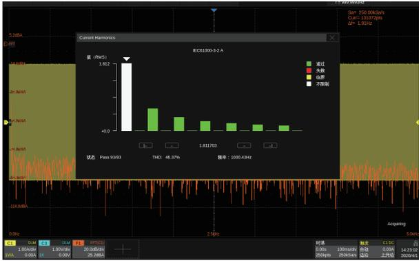
The Power Analysis option provides a full suite of power measurements and analysis, which greatly improves the measurement efficiency in switching power supplies and power devices design
