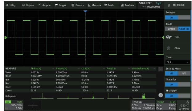
Parameter measurements includes 4 categories: Vertical, Horizontal, Miscellaneous and Channel Delay providing a total of 50+ different types of measurements. Measurements can be performed within a specified gate period. Measurements on Math, Reference and History frames are supported.
