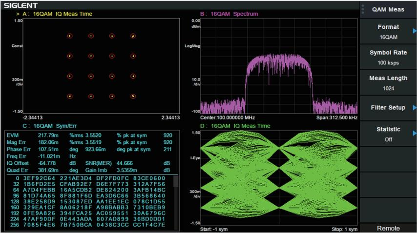
The SDG6000X supports popular modulation types such as ASK, FSK, PSK, and QAM. Proprietary resampling technology provides excellent EVM performance at arbitrary symbol rates between 250 Symb/s ~ 37.5 MSymb/s. Built-in digital quadrature modulator provides the possibility to generate IQ signals from baseband to 500 MHz intermediate frequency.
